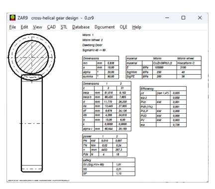
ZAR9 calculates dimensions and load-bearing capacity of helical gears with crossed axis. Axis angle may be 90 degrees or any other input value. Sum of helical angle of the gear pair is axis angle. For example, it may be a screw gear with 45+45 degrees, or a worm and worm wheel with 80+10 degrees. ZAR9 calculates efficiency, forces and safety against sliding abrasion, tooth root breakage and seizure.
