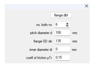
Entering the dimensions of the inner, outer and bolt circle diameter of the circular flange is now easier by simply selecting circular flanges according to EN 1092-1 from the database in sizes PN 6 to PN 100.
