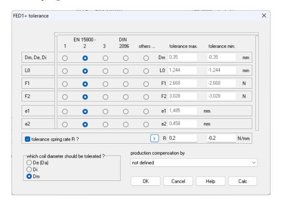
In FED1+ you can optionally enter a tolerance for the spring rate R. A value is suggested with the "<" button. The question is asked again and again how this default value is determined:
