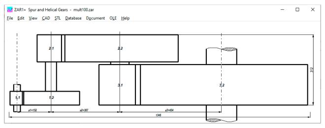
When pre-designing multi-stage gears, the most important dimensions have been added to the drawing: center distances between the stages, overall length, overall width.
