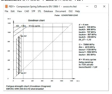
The oil tempered spring steel wires SWOSC-V according to the Japanese JIS standard and SWOSC-VHV are comparable with VD-SiCr and VD-SiCrV according to EN 10270-2. The two materials were added to fedwst.dbf, the technical data was taken from Suzuki-Garphyttan and is similar to Oteva70 and Oteva75.
