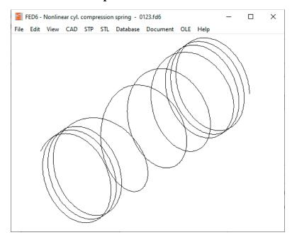
Just like in FED1+, FED3+, FED5, FED17, you can now also export the center line of the spring as a 3D helix in STP format in FED6 and FED7 and transfer it to CAD. To represent a 3D spring, you can then extrude the wire around the helix in the CAD program and cut off the spring ends (in the case of ground spring ends).
