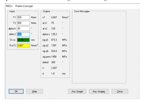
In the pre-design or in the design basic data or in the design quick input, the entered spring angle delta2 was changed for the calculation method R = 1/(1/R0+1/RS1+1/RS2) and for supported springs with bent legs and a large lever arm. Now only the coil diameter is adjusted when changing the input data.
