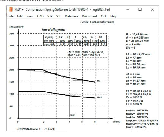
UGI 202N is an austenitic stainless, non-magnetic steel with a high manganese content (X8CrMnNiN18-9-5) and has been added to the materials database. Fatigue strength values are not available.
