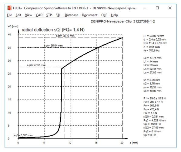
The transverse spring rate goes to 0 and remains 0 from s = sk, when the spring buckles. The transverse force curves are interesting. If the spring does not buckle, the transverse spring rate may both increase or decrease, or both, depending on the distance to the buckling area.
