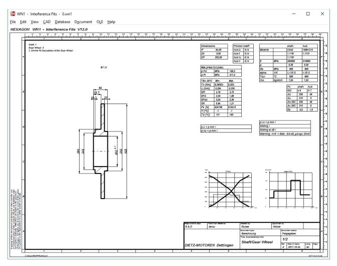
New Quick2 View provides a quick overview about calculation results and dimensions of the joint.
