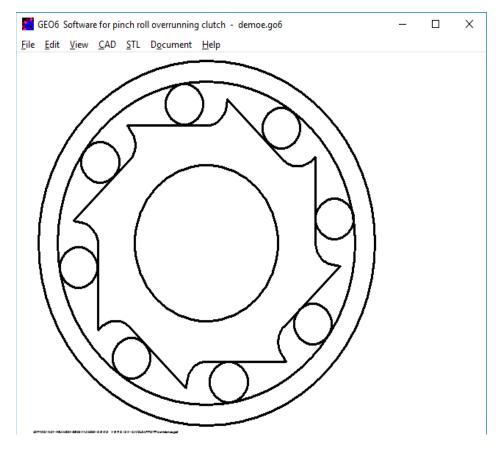
Geometry of inner ring and outer ring is generated by GEO6.
