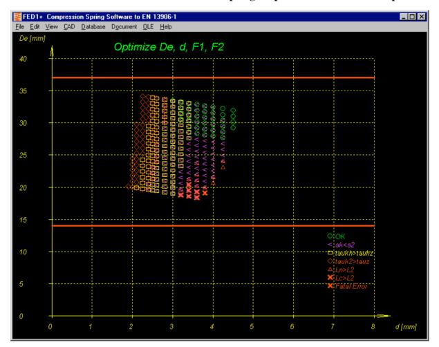
FED1+: Point cloud as result of search run for springs in pre-defined installation space
