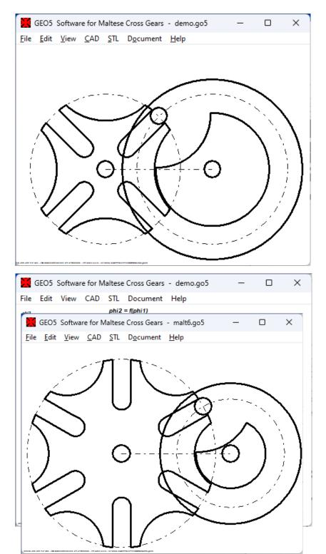
**Calculation and Design of Geneva mechanism** GEO5 calculates dimensions, operation angle, velocity and acceleration of Maltese cross gears. GEO5 generates drawings of Maltese cross wheel and driving wheel as DXF or IGES files to be used with your CAD software. The component parts can be generated as STL files, then printed on a 3D printer and assembled as functioning model of a Geneva mechanism.
